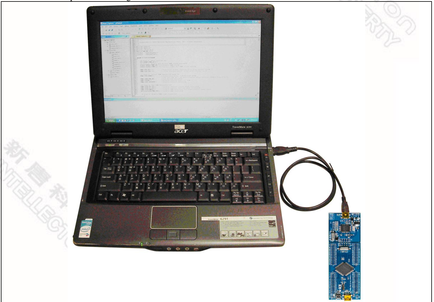
Figure 4-1 NuTiny- SDK-NUC140 Hardware Setup
