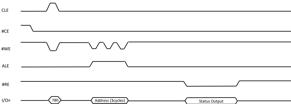
Figure 9-11 Read Status Enhanced (78h) Operation
