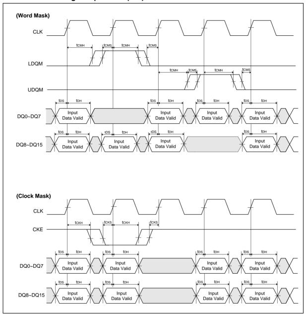
10.4 Control Timing of Output Data (x16)
