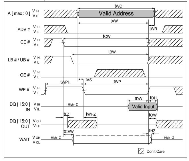
10.2.17 Asynchronous WRITE Using ADV#
