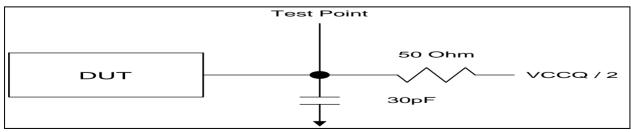
Note: All tests are performed with the outputs configured for default setting of half drive strength (BCR[5:4] = 01b).
