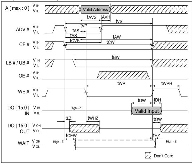
10.2.18 Burst WRITE Operation-Variable Latency Mode
