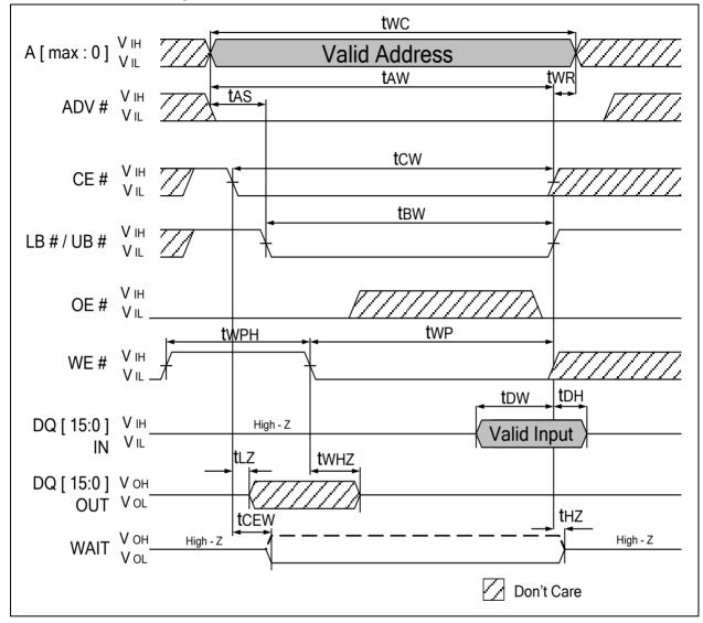
10.2.16 WE# - Controlled Asynchronous WRITE
