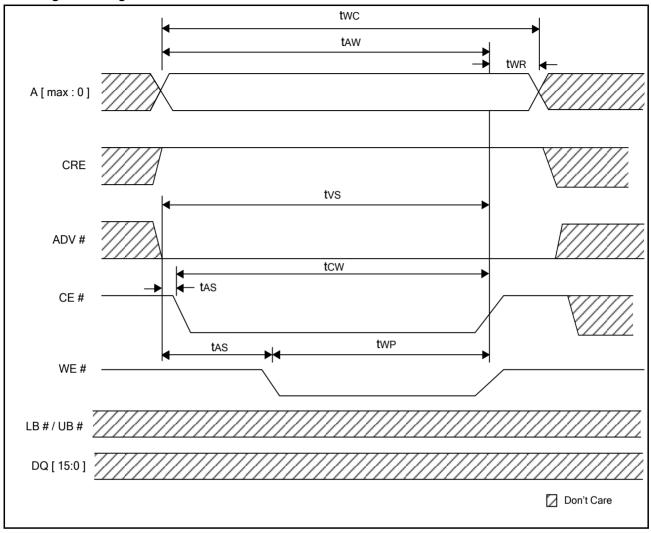
8.4.1.3 Configuration Register WRITE, Synchronous Mode Followed by READ ARRAY Operation
