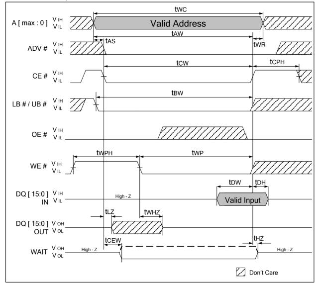
10.2.15 LB# / UB# Controlled Asynchronous WRITE
