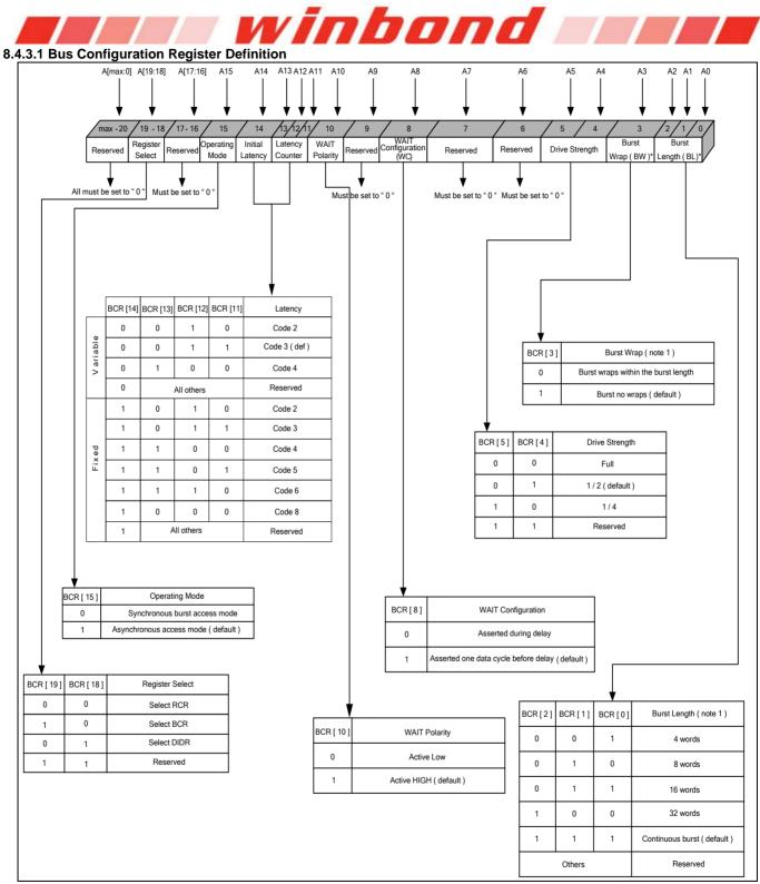
Note: 1. Burst wrap and length apply to both READ and WRITE operations.
