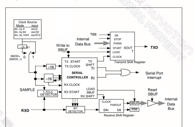
Figure 22. Serial Port Mode 2
