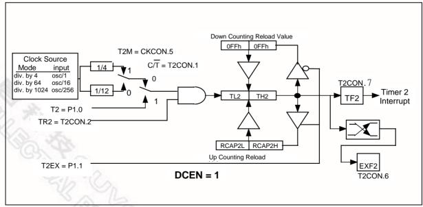
Figure 16. 16-Bit Auto-reload Up/Down Counter
