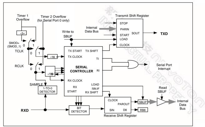
Figure 21: Serial Port Mode
