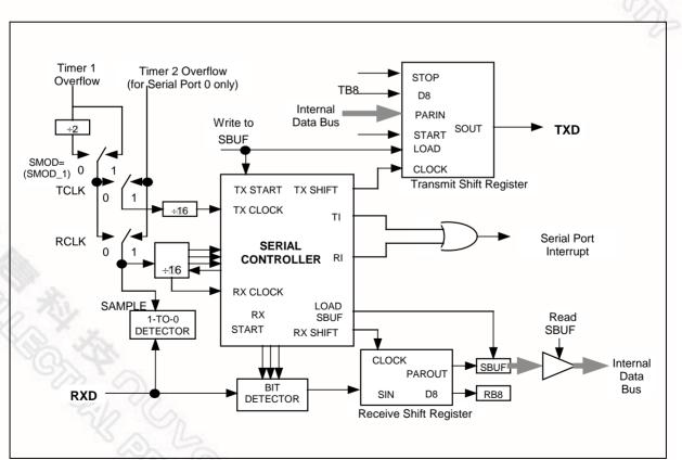
Figure 23: Serial Port Mode 3
