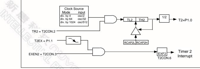
Figure 18. Programmable Clock-Out Mode
