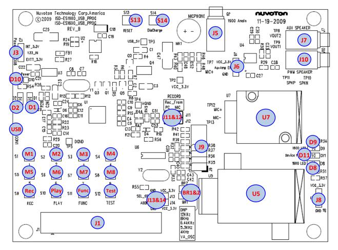
Figure 3-1 ISD-ES1900\_USB\_PROG Rev-B Top View Components
