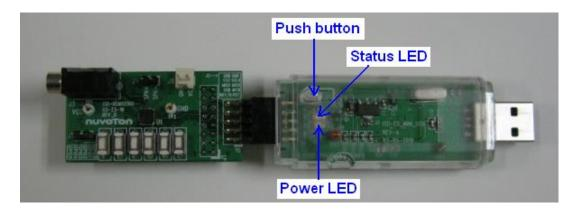
Figure 7 – Power LED, Status LED and Push button
