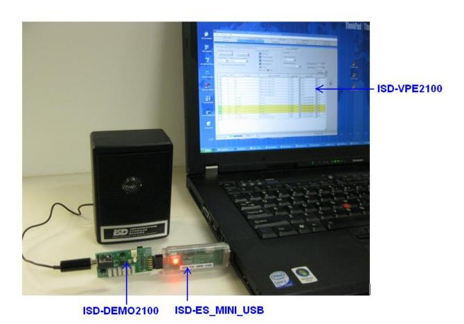
Figure 4 – A complete evaluation environment for ISD2100 device
