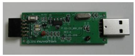
Figure 1 – Top view of ISD-ES\_MINI\_USB board
