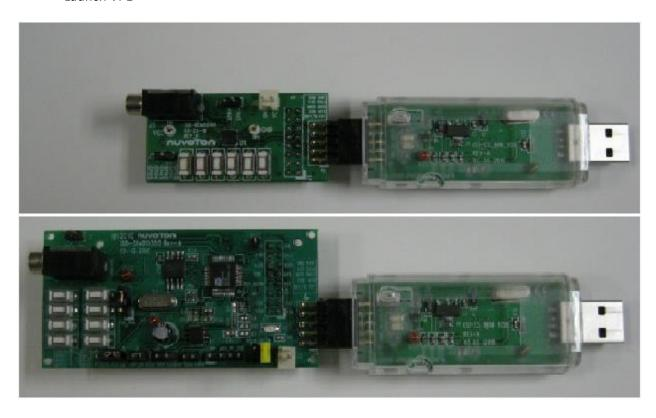
Figure 5 – To connect demo board and USB dongle: top side face up for both boards.
