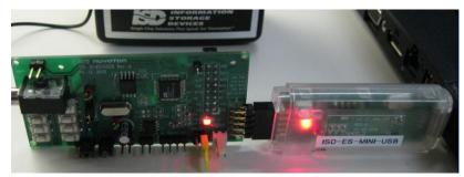
Figure 6 – USB dongle connected with ISD-DEMO15D00
