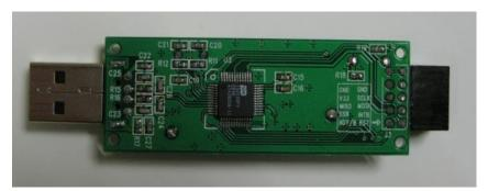
Figure 2 – Bottom view of ISD-ES\_MINI\_USB board
