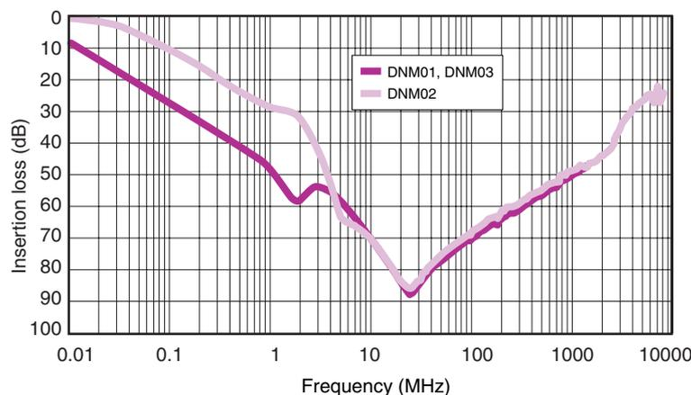
**COMPLEX STYLE EMI FILTERS · BLOCK TYPE EMI FILTERS [ DNM Series ]**
