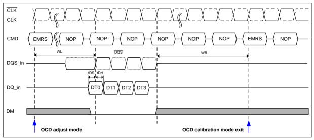
Figure 7 - OCD Adjust Mode
