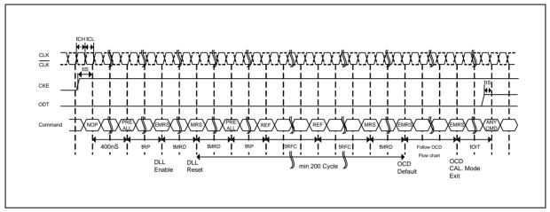
Figure 1 - Initialization sequence after power-up
