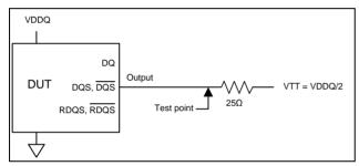
Output slew rate test load
