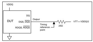
Figure 16 - AC timing reference load
