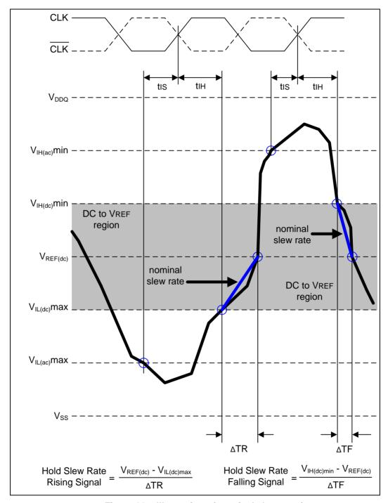
Figure 22 - Illustration of nominal slew rate for tIH
