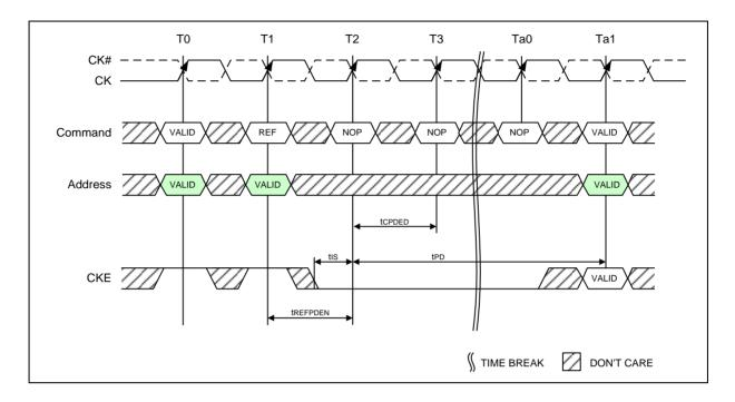
Figure 65 - Refresh Command to Power-Down Entry
