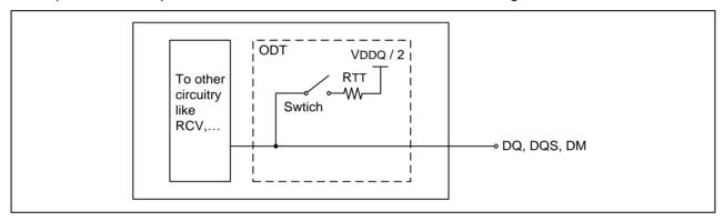
Figure 73 - Functional Representation of ODT
