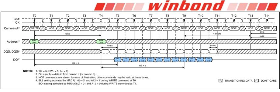
Figure 53 - WRITE (BL8) to WRITE (BC4) OTF
