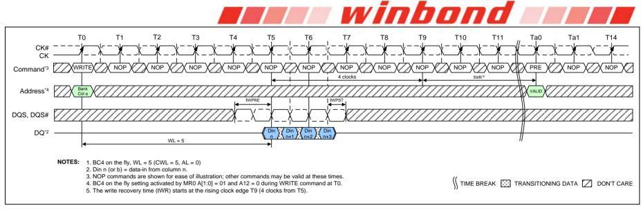
Figure 47 – WRITE (BC4) OTF to PRECHARGE Operation
