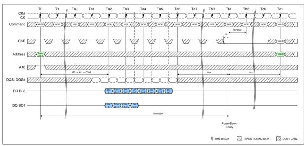
Figure 62 - Power-Down Entry after Write
