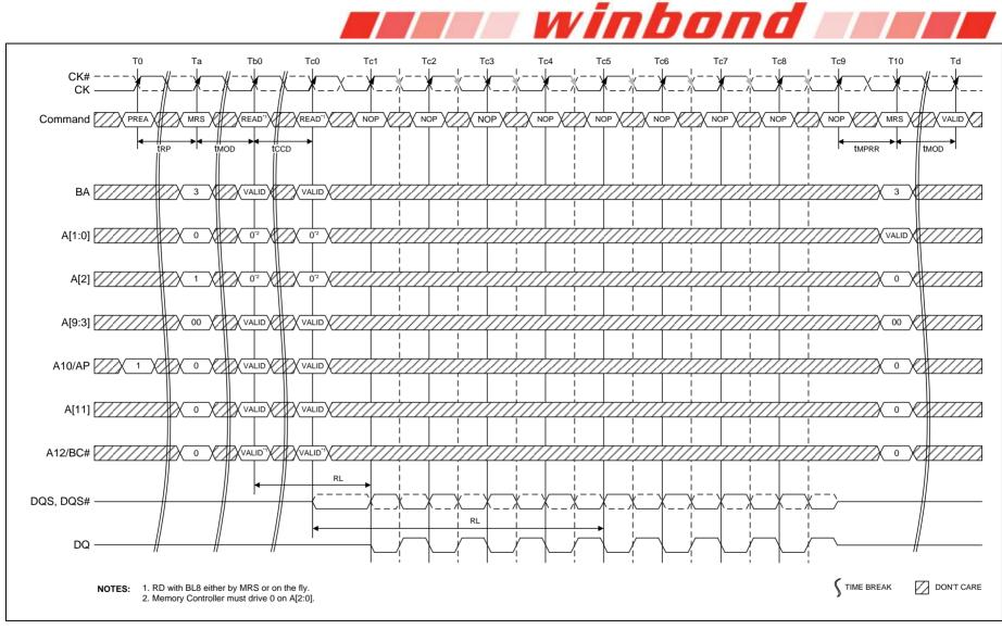
Figure 18 - MPR Readout of pre-defined pattern, BL8 fixed burst order, back-to-back readout
