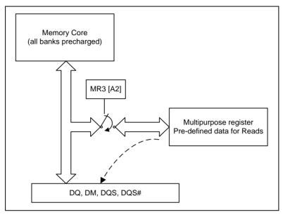
Figure 16 - MPR Block Diagram
