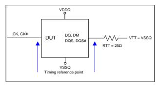
Figure 98 - ODT Timing Reference Load
