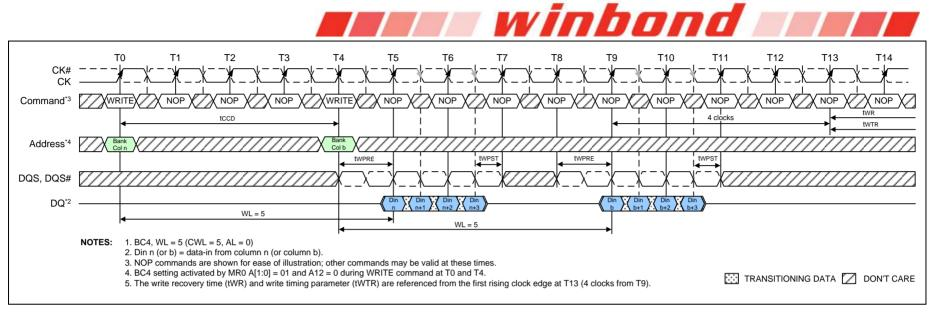
Figure 49 - WRITE (BC4) to WRITE (BC4) OTF
