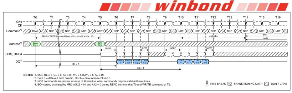
Figure 33 - READ (BC4) to WRITE (BC4) OTF
