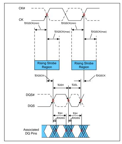
Figure 23 - READ Timing Definition
