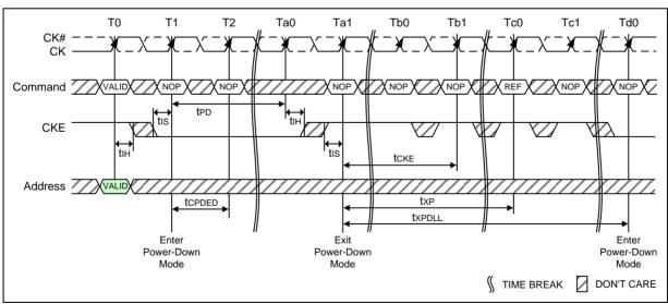
Figure 70 - Power-Down Entry/Exit Clarifications - Case 2
