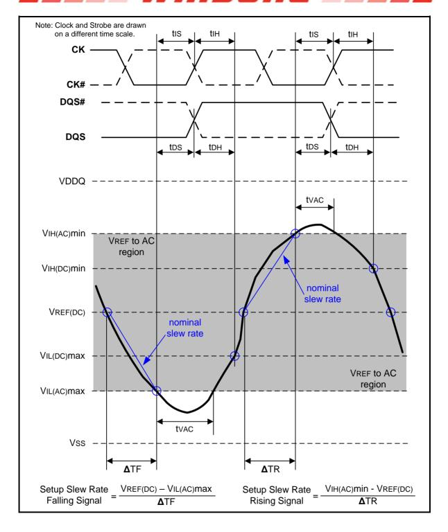
Figure 107 – Illustration of nominal slew rate and tVAC for setup time tDS (for DQ with respect to strobe) and tIS (for ADD/CMD with respect to clock)
