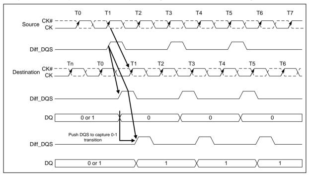
Figure 13 - Write Leveling Concept
