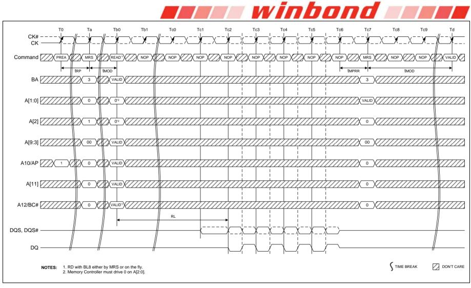
Figure 17 - MPR Readout of pre-defined pattern, BL8 fixed burst order, single readout
