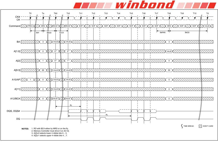
Figure 19 - MPR Readout pre-defined pattern, BC4, lower nibble then upper nibble
