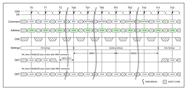
Figure 3 - tMRD Timing
