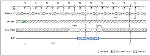
Figure 45 - WRITE (BC4) to READ (BC4) Operation
