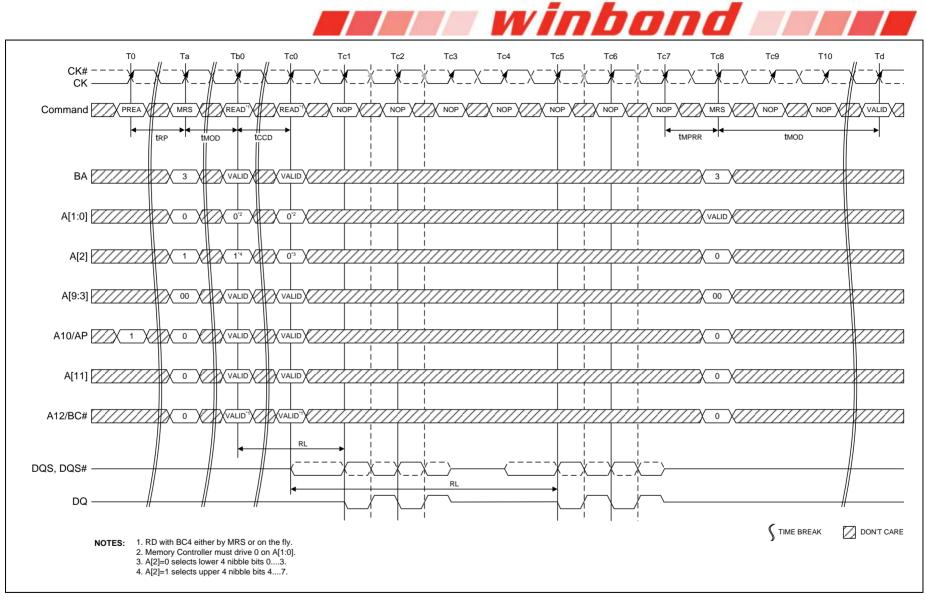
Figure 20 - MPR Readout of pre-defined pattern, BC4, upper nibble then lower nibble
