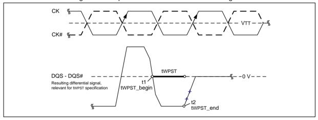
Figure 42 - Method for calculating twpst transitions and endpoints
