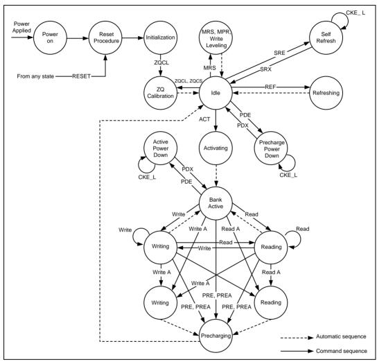
Figure 87 – Simplified State Diagram
