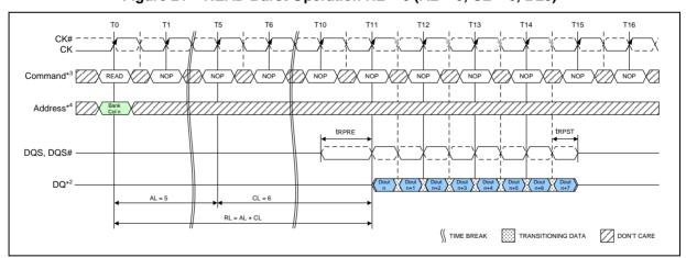
Figure 21 - READ Burst Operation RL = 6 (AL = 0, CL = 6, BL8)
