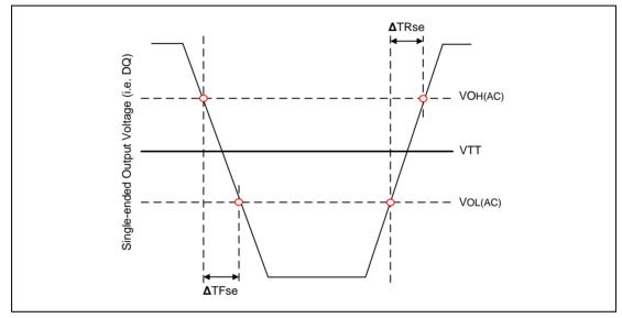
Figure 94 - Single-ended Output Slew Rate Definition
