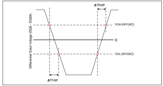
Figure 95 - Differential Output Slew Rate Definition
