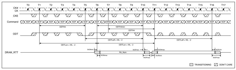
Figure 75 – Synchronous ODT (BL = 4, WL = 7)
