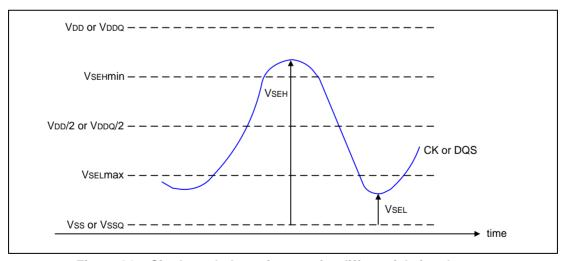
Figure 91 - Single-ended requirement for differential signals
