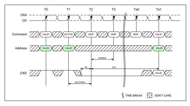
Figure 66 - Active Command to Power-Down Entry
