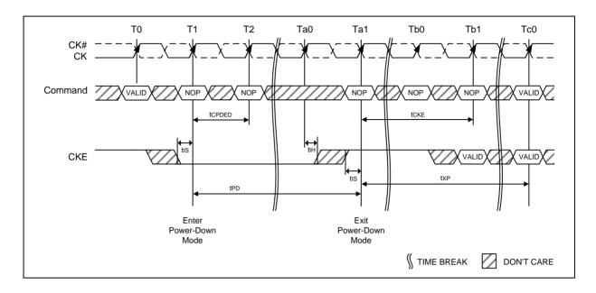
Figure 63 - Precharge Power-Down (Fast Exit Mode) Entry and Exit
