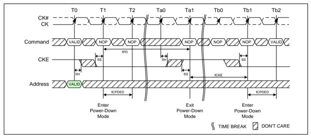
Figure 69 - Power-Down Entry/Exit Clarifications - Case 1
