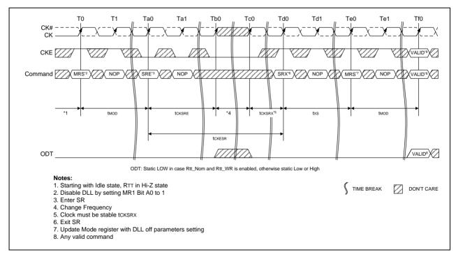
Figure 10 - DLL Switch Sequence from DLL-on to DLL-off
