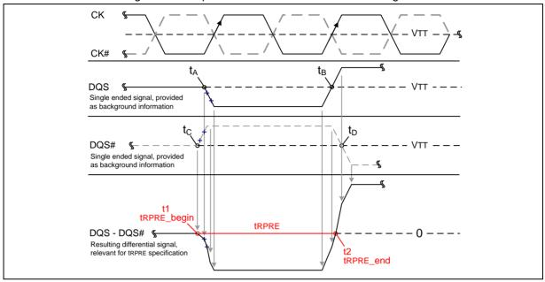
Figure 27 - Method for calculating tRPRE transitions and endpoints
