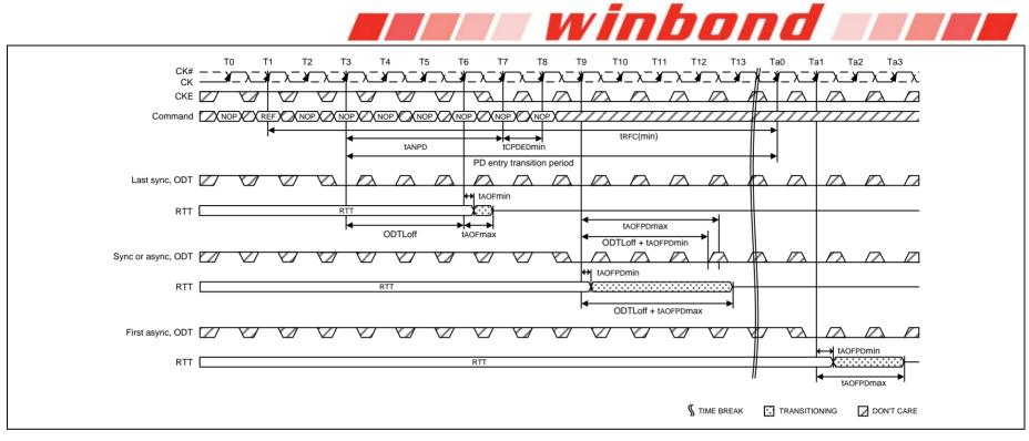
Figure 84 – Synchronous to asynchronous transition after Refresh command (AL = 0; CWL = 5; tanpo = WL - 1 = 4)
